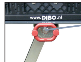
19mm screw to adjust length of the support arm
